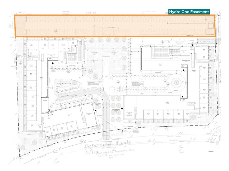
**The Alternate Parking Plan** shown above utilizes the Hydro One easement (corridor) on the north end of the site to increase surface parking and reduce the size of the underground parkades to the footprints of the buildings and their respective interior courtyards.
